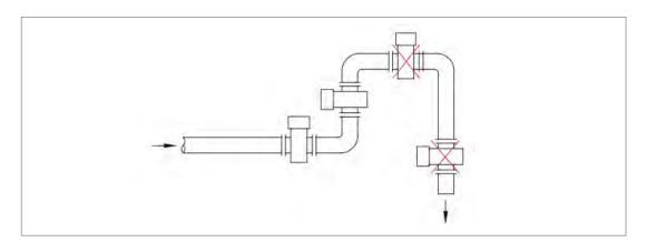
Install flow meter at the rising pipe
