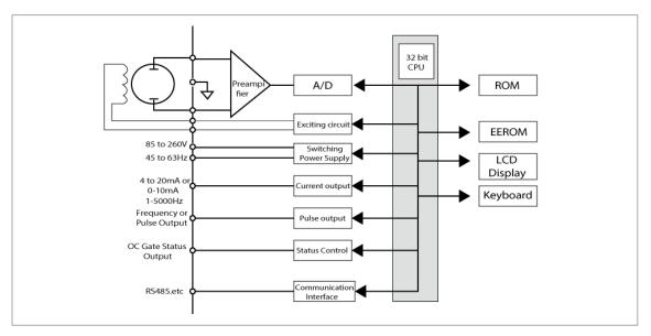
The converter can supply the exciting current to the coil in the sensor of electromagnetic flow meter; the head amplifier amplifies the electromotive force from the sensor and converts it into standard signals of current or frequency so that the signals can be used for displaying, controlling, and processing.
