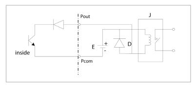
Commonly, the relay needs E as 12V or 24V. D is an extended diode, most middle relays now have this diode inside. If not have, the user can connect one outside.
