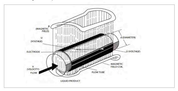
Operation of an Electromagnetic Flow Meter
