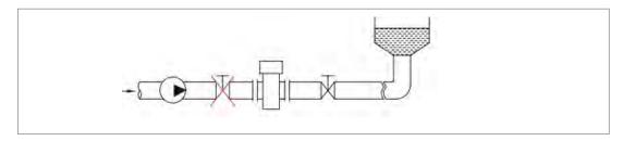
• Sensor should be installed at the outlet of pump and not at the inlet
