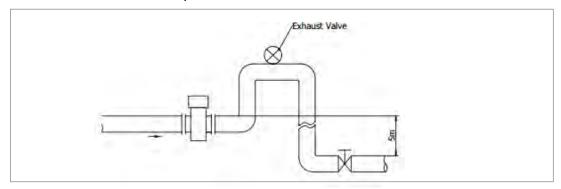
• Control valve and stop valve should be installed at the downstream of sensor and not at the upstream side.
