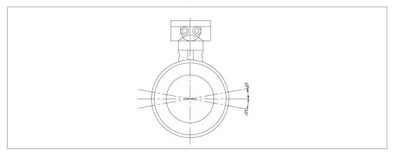
At flow meter upstream, there should be straight pipe no less than 5D and no less than 2D at flow meter downstream. (D is the inner diameter of the flow meter)
