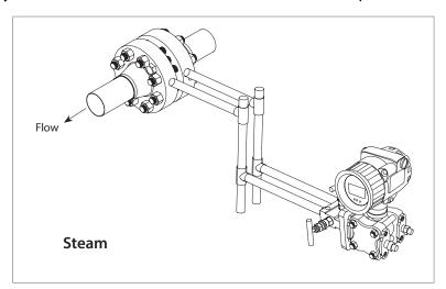
**Note:** For steam or other elevated temperature services, it is important that temperatures at the process connection do not exceed the transmitters process temperature limits.
