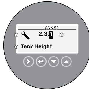
Fig 48: Local display screen layout in configuration mode
