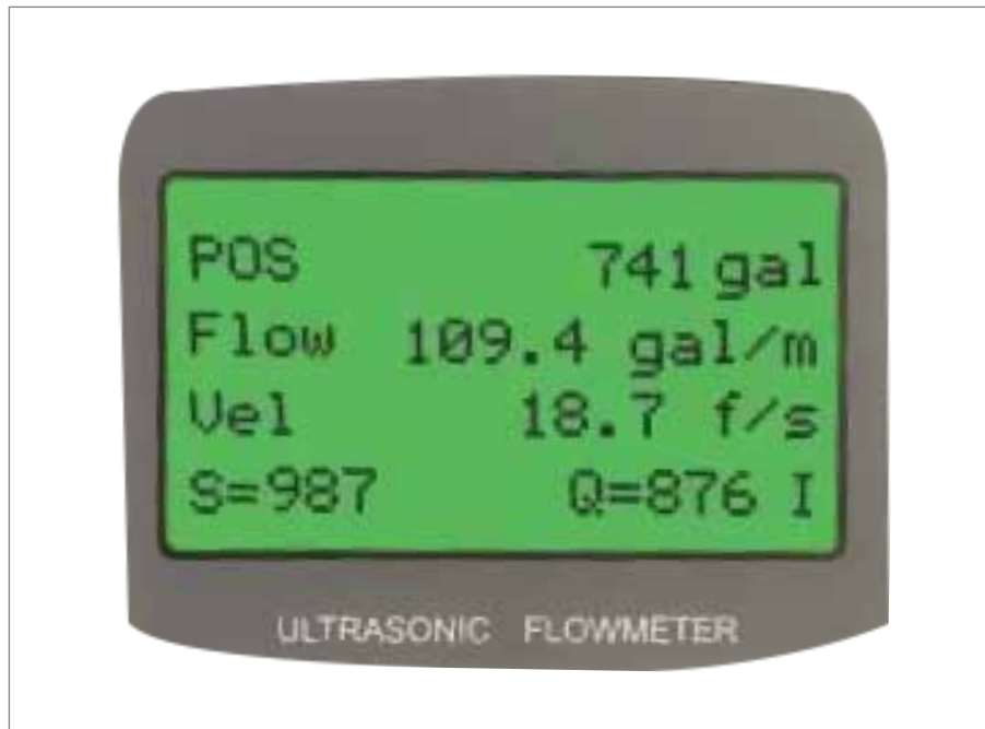
Fig 7: Display for Tek-Clamp 1200A-100H Handheld Ultrasonic Flow Meter
