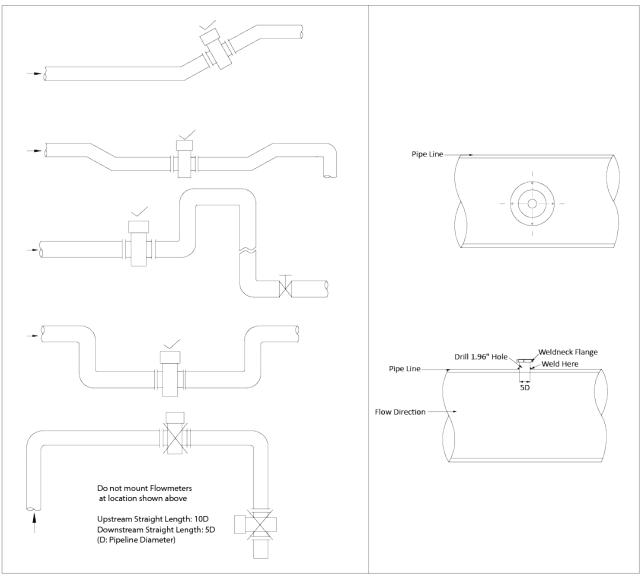
At flowmeter upst ream, there should be straight pipe no less than SD and no less than 2D at flowmeter downstream. (D is the inner diameter of flowmeter)
