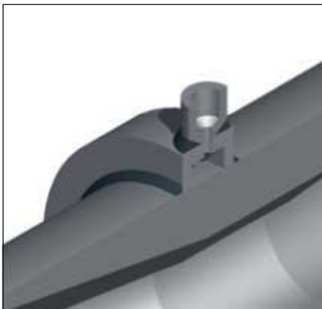
Fig 14: Annular Chamber Tap with Welded Ring
