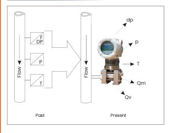
The Tek-Bar 3800XH/A Multivariable Transmitter measures differential pressure, static pressure (absolute or gauge), and process temperature. It also performs flow calculations, compensating for pressure or temperature and accounting for variables such as discharge coefficient, thermal expansion, Reynolds number, and compressibility factor.
