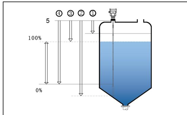
**Note:** The level of the measured medium must not be in either the blanking zone.
