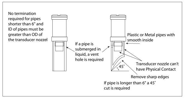
Stilling Well must be within 5" of the bottom of the tank with 45° cut.
