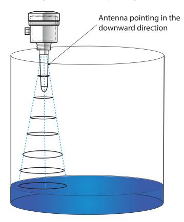
Note: Tek-Wave 4300A can only be mounted on metal tanks
