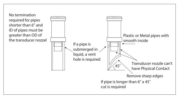
Stilling Well must be within 5" of the bottom of the tank with 45° cut.
