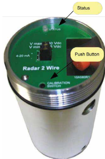
Fig 26: The illustration shows the location of the LED and the push button for Radar sensors.
